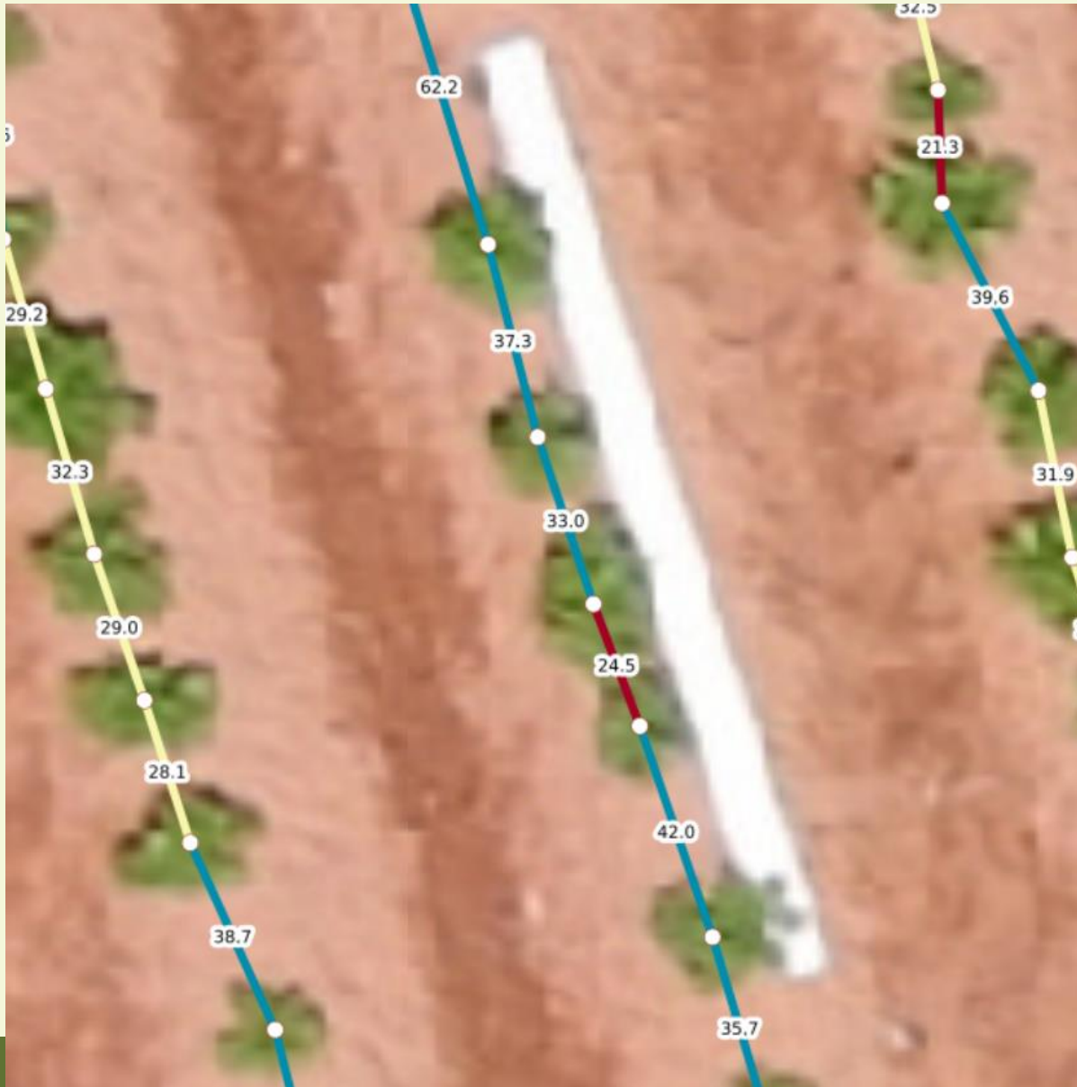
Plant Spacing (cm) - In-situ measurement vs Drone based measurement
